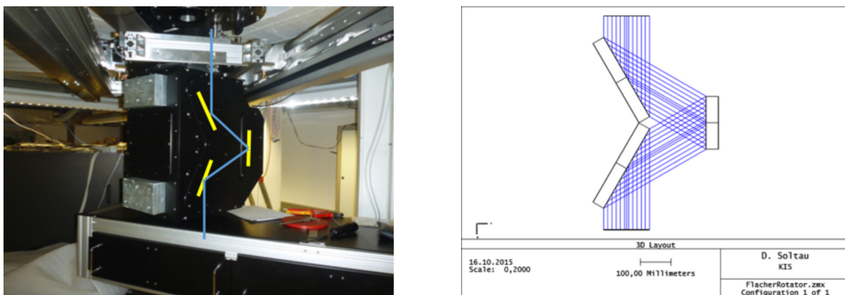
Fig. 1: Left: Derotator as installed at GREGOR with its light path indicated. Right: Zemax model (from D. Soltau).
