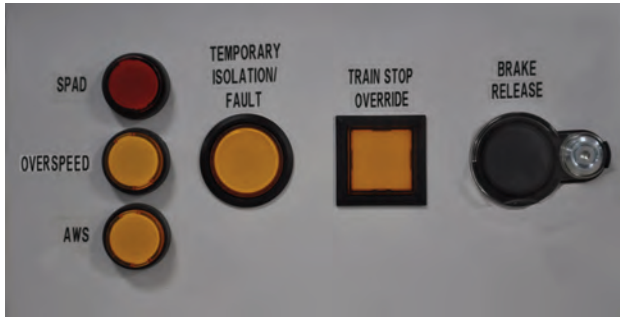
Example of enhanced TPWS control panel
