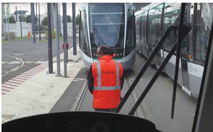
▲ ABOVE: Parisian operator RATP carried out a pilot with 'driverless' tram stabling in conjunction with Alstom in 2017. A retrofitted Citadis manoeuvred itself around the T7 depot in Vitry-sur-Seine, following staff members around at safe distances and stopping at designated stabling positions. RATP/Alstom
