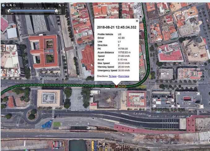
A ABOVE AND RIGHT: Simple graphical interfaces give valuable real-time information of all vehicles in current operation. This data helps enhance safety and efficiency while improving training regimes and reducing cost. MetroTenerife
