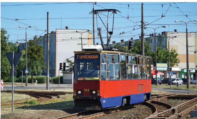
▲ ABOVE: An early Pesa venture in the tram market, this 2003 Konstal 805Na remodelling created the only examples of type 805Nm , allocated numbers 362 and 363.
