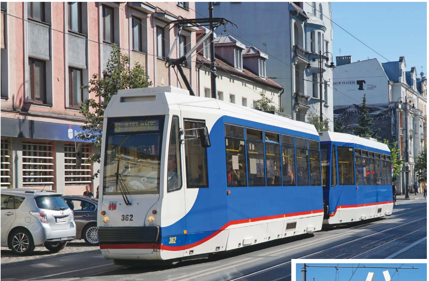
▲ ABOVE: An early Pesa venture in the tram market, this 2003 Konstal 805Na remodelling created the only examples of type 805Nm , allocated numbers 362 and 363.
