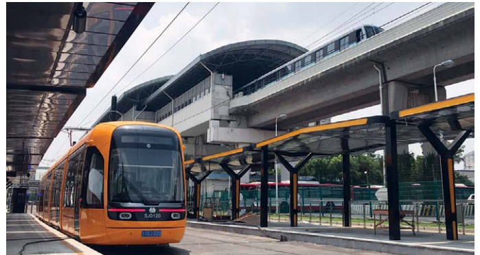
▲ One of the first batch of Alstom Citadis trams for Shanghai stands at the Songjiang South interchange terminus between the new tramway and metro line 9. Keolis
