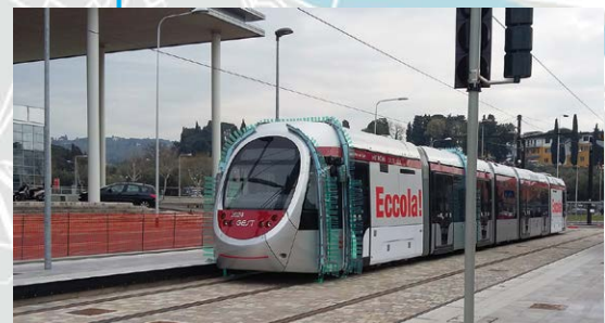
▲ Tram 2024 at Careggi terminus in March 2018 on gauging tests. The sign on the side translates to 'Here it is!'. A Fantechi
