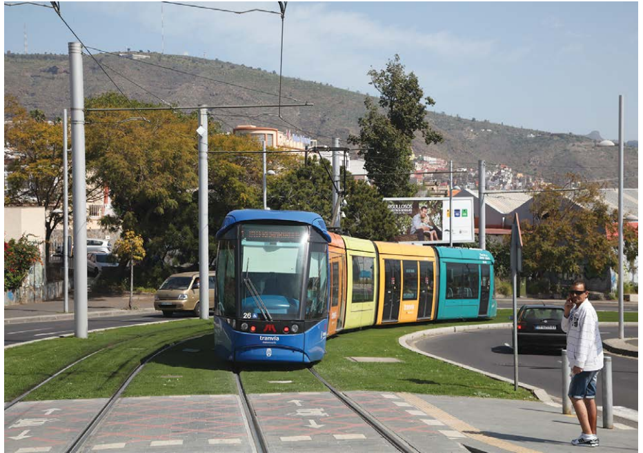
▲ Metrotenerife Citadis 26 taking the curve below Conservatorio stop heading to Santa Cruz; its SIMOVE system was developed in response to over-speeding incidents on curves on a variety of networks. Mike Russell
