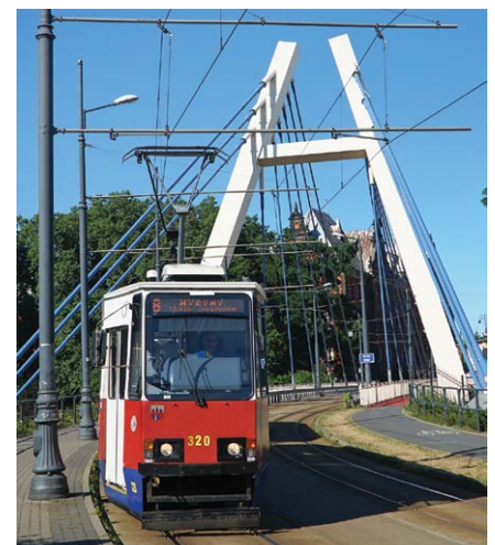
▲ ABOVE: An early Pesa venture in the tram market, this 2003 Konstal 805Na remodelling created the only examples of type 805Nm , allocated numbers 362 and 363.
