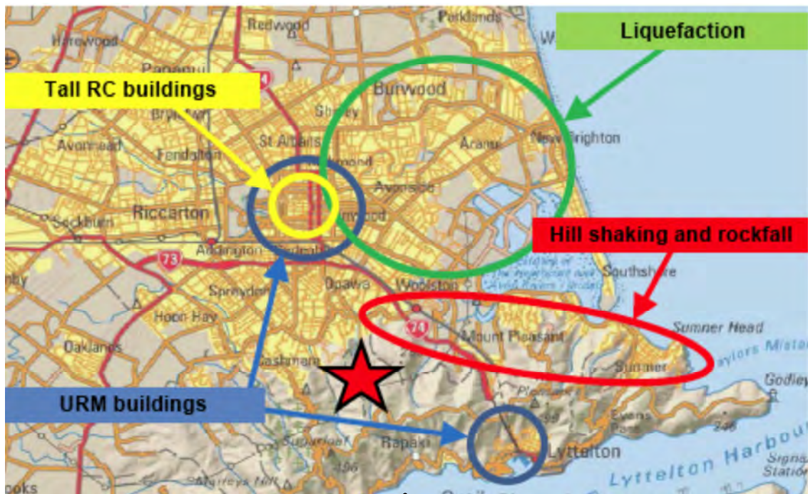
Damage from 22 Feb 2011 Christchurch earthquake 3
