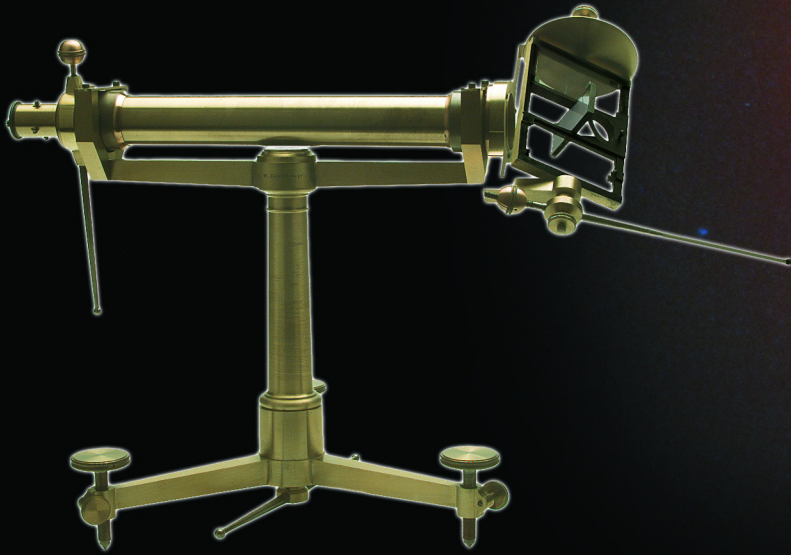
Figure 1 The first heliotrope instrument made for Gauss by Breithaupt of Kassel, Germany. Photo courtesy Hans-Helmut Breithaupt.
