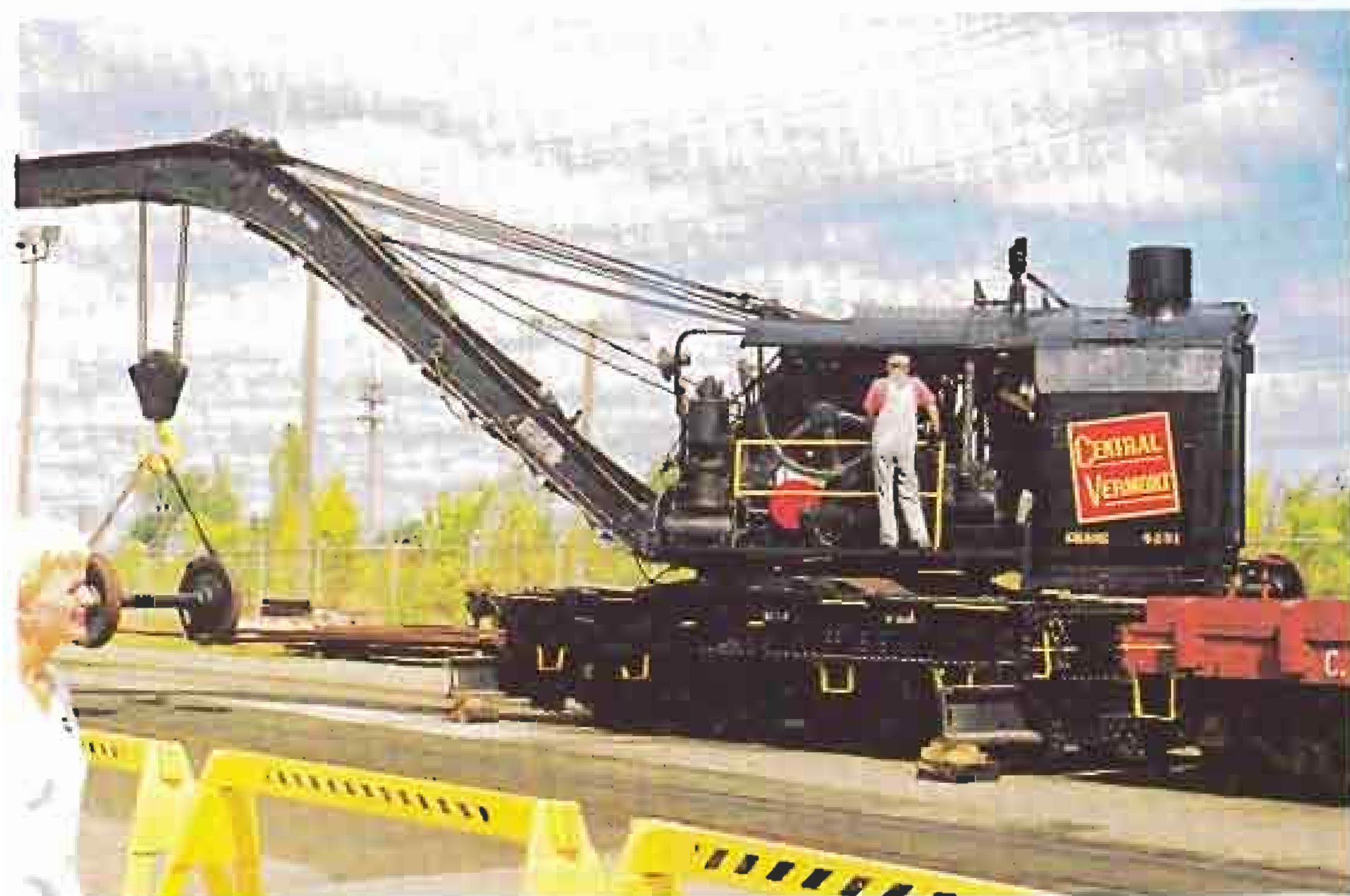
The Bytown Railway Society's ex-Central Vermont 1919-built Industrial Brownhoist 50-Ton steam crane 4251 performs for guests at the Canada Science & Technology Museum on September 1. Photo by Paul Bown.
