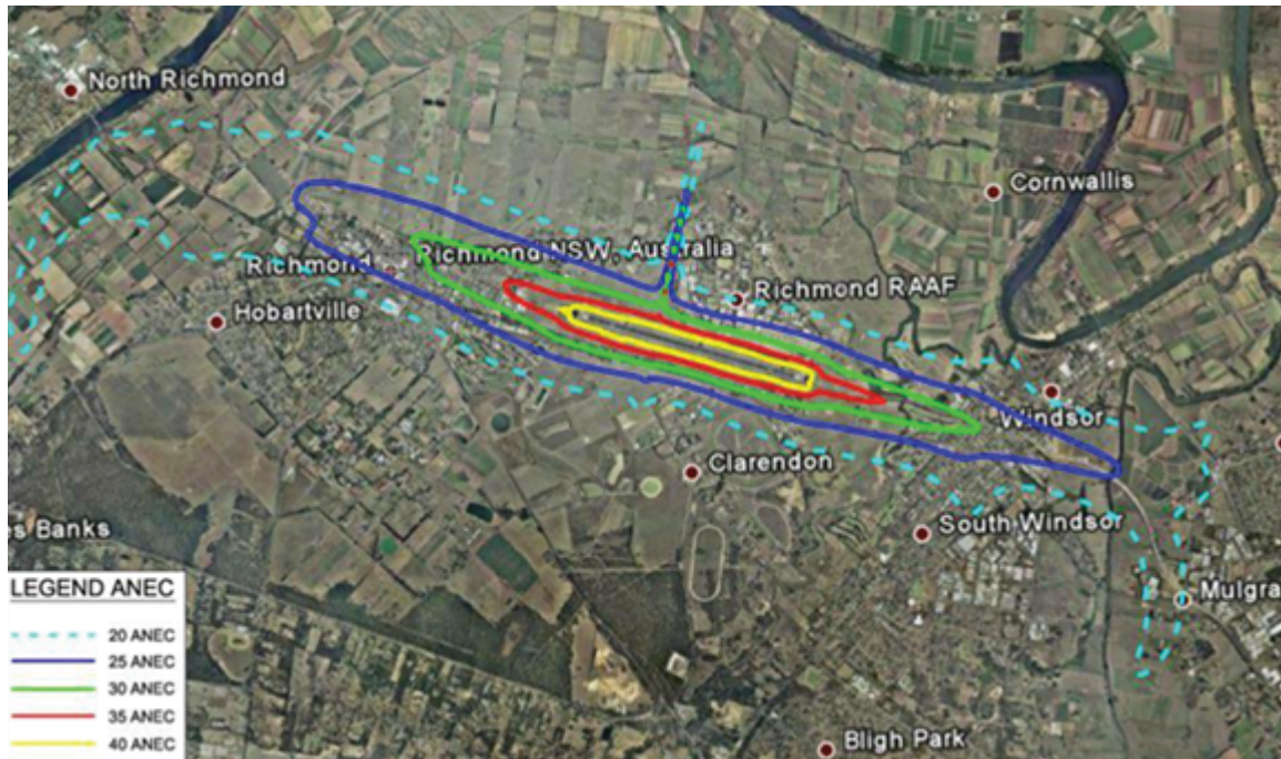
Figure 130 ANEC contours expected for a Richmond east-west layout supporting one million passengers
