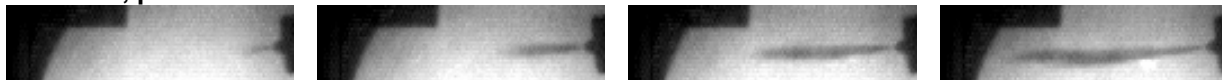
Figure 5. Spray evolution inside the vessel (inj. pressure: 600 bar, energ. time: 600 \mu s).
