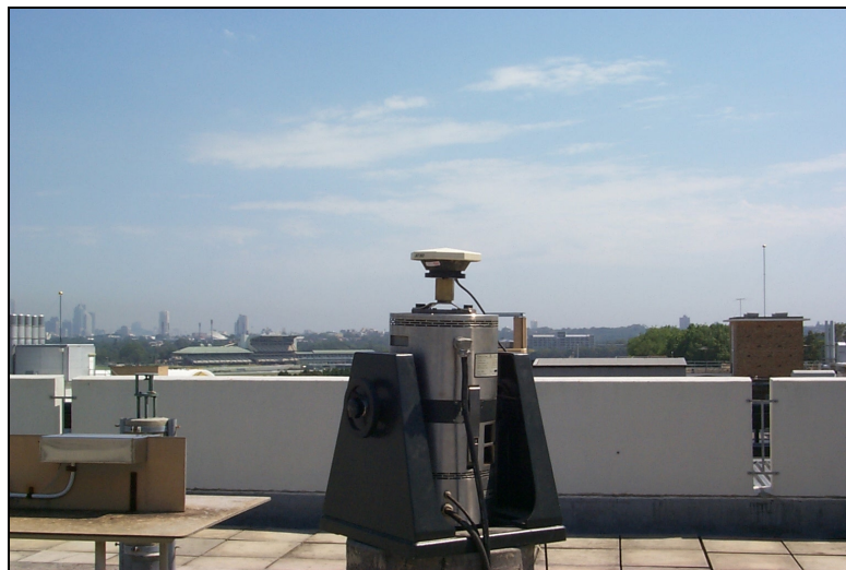
Figure 7.1. The experiment at UNSW (24th January 2001) -- The 'rover' antenna atop the mechanical shaker
