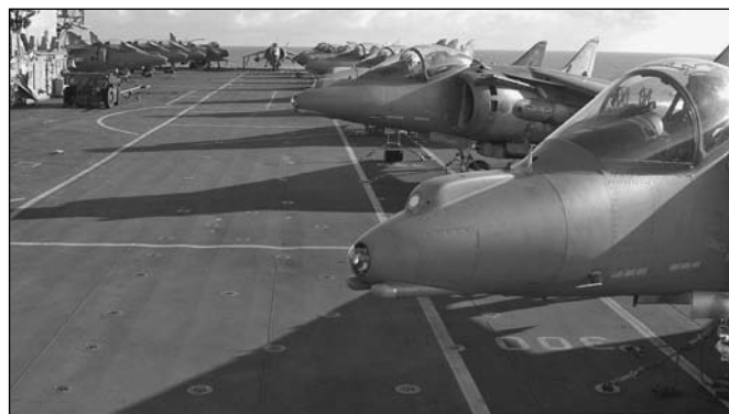
The Joint Force Harrier concept in practice. RN Sea Harriers and RAF GR-7 Harriers on the deck of HMS ILLUSTRIOUS. The RAF aircraft have more powerful engines and can thus operate in areas of high temperature that the Sea Harrier cannot. They are also more upgradeable than the Sea Harrier. (RN)
