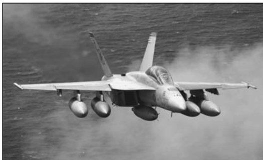
An F/A-18F Super Hornet with four large fuel tanks and a buddy refuelling pod on the centreline. Australia will get 24 Block II Super Hornets by 2010 to replace the F-111. (USN)
