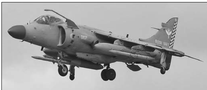
An improved FA-2 Sea Harrier in the hover. The FRS-1 Sea Harrier underwent an improvement to include the new Blue Vixen radar in the modified nose, which enabled the use of the AIM-120 AMRAAM.
