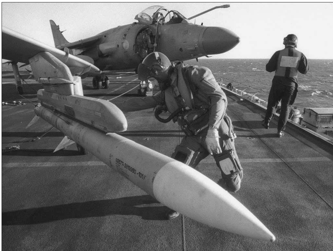
A Sea Harrier pilot checks his AIM-120 AMRAAM before take off. With the addition of the Blue Vixen radar and AMRAAM the Sea Harrier was, for a while, the best air superiority fighter in Europe.
