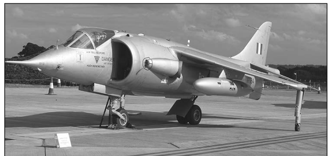
A P1127 Kestrel. The P1127 was the first 'jump jet'. Test and evaluation would later spur on development of the RN Sea Harrier and RAF GR series of Harrier.
