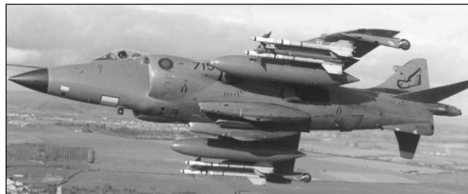
The Sea Harriers sent to the Falklands after the war on HMS ILLUSTRIOUS were modified with double racks of AIM-9L Sidewinder and larger external fuel tanks. These improvements provided longer range and time on station as well as twice the fire power.
