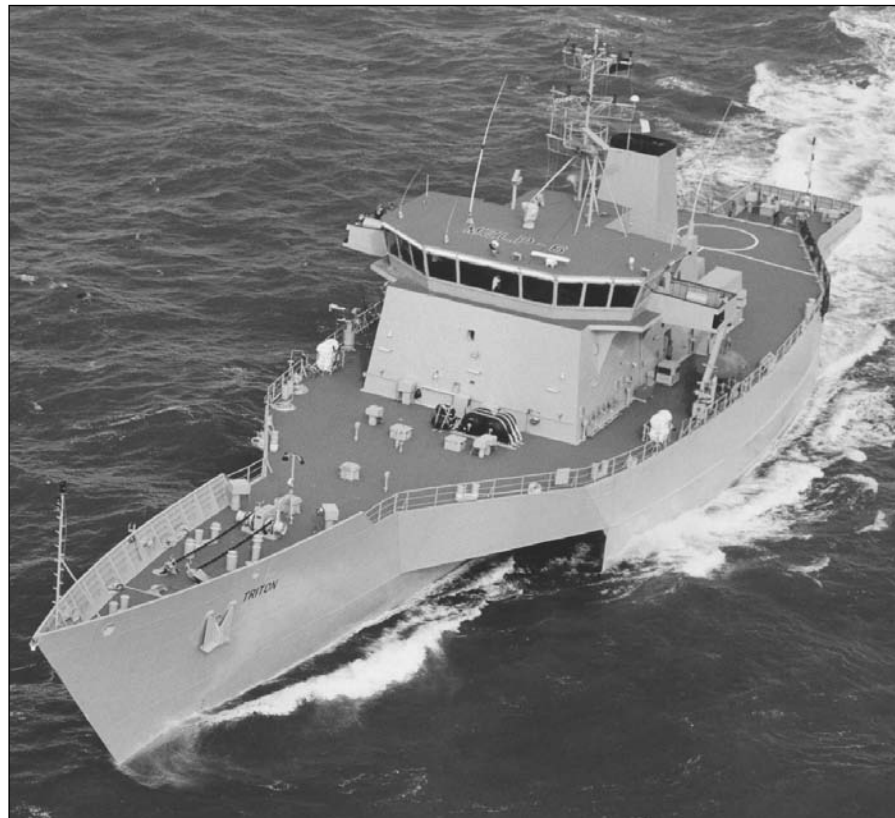
Australia's latest border protection weapon against illegal foreign fishing is the ACV Triton . Originally built to investigate trimaran warship designs for the RN, the vessel will now ply Australian waters till 2008.
