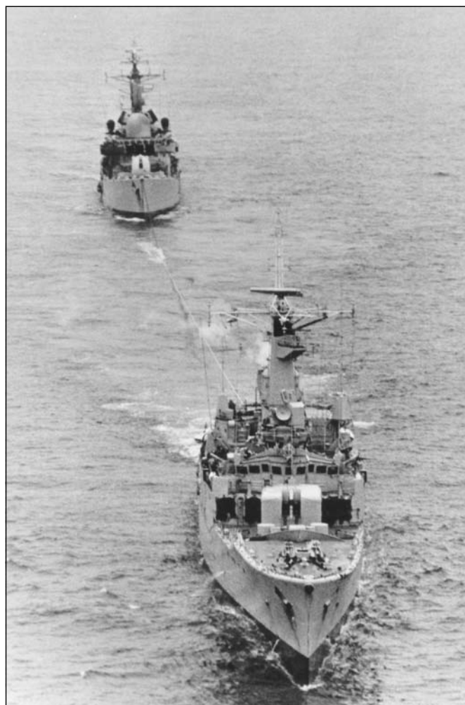
The frigate HMS YARMOUTH towing the abandoned SHEFFIELD to South Georgia. With a large amount of fire fighting water still present and a large hole in her side SHEFFIELD sank on route to South Georgia when water flooded in through the hole during a storm. (RN)
