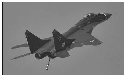
A Russian Navy MiG-29K during a test flight with arrestor hook down.
