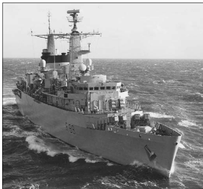
The Type 22 frigate BROADSWORD. Only two Type 22 frigates were available to the Task Force. Their main role was to defend the carriers from Exocet attack given their accurate Sea Wolf missile system. (RN)
