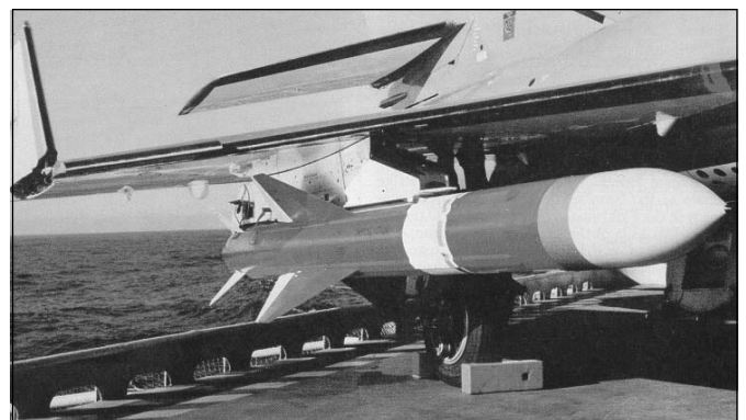
An AM-39 Exocet ASM under the wing of a Super Etendard. Argentina tried to buy Exocets on the Black Market but were unsuccessful.
