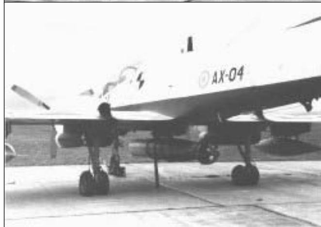
Three images of the test aircraft evaluating the Mk-13 torpedo. The torpedo can be seen on the centreline pylon. It was never used.
