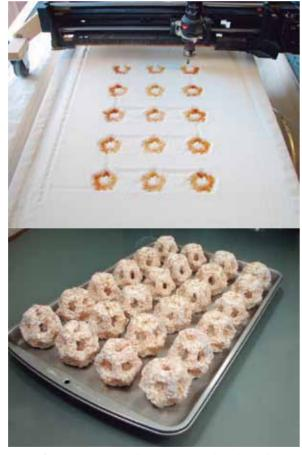
Manufacturing process with an experimental machine where the raw material is sugar. CandyFab 4000 by Evil Mad Scientist Laboratories.
