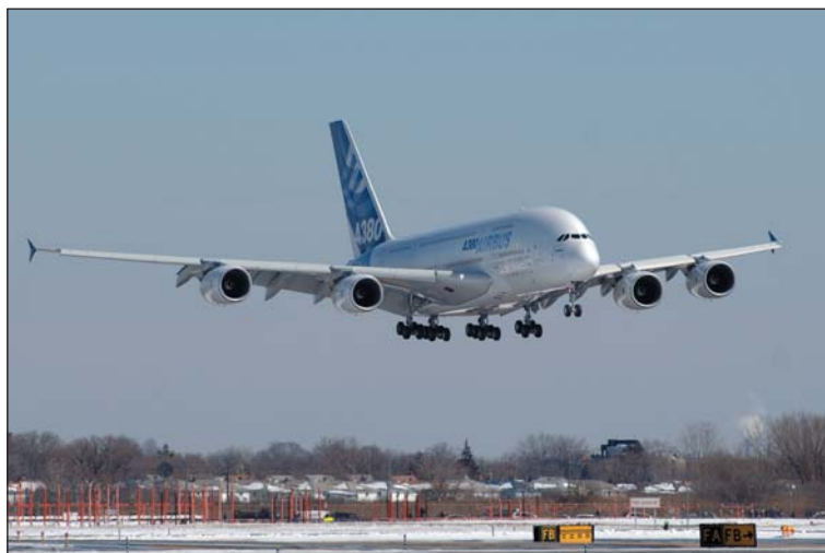
The Airbus A380 is a double-deck, four-engine airliner that can carry 555 passengers. It is the largest passenger airliner in the world, with a length of 240 feet and a wingspan of 262 feet. Image courtesy Airbus.
