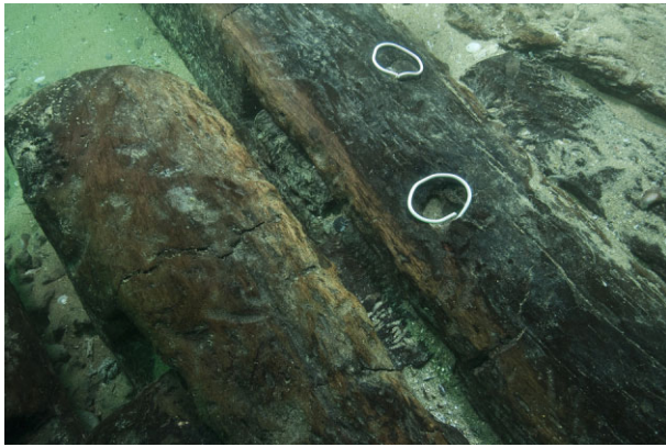
Figure 24. Two tenon-ribs pegged in a double-width channel at the stern area of Ship 17 (port strakes P3 and P4). (Photo by Christoph Gerigk © Franck Goddio/Hilti Foundation)
