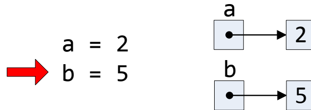
Figure 2.3 How variable bindings change as a program runs: step 2
