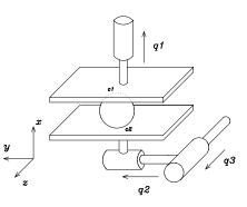
Figure 3: A schematic of the "dextrous gripper" of the University of Pisa
