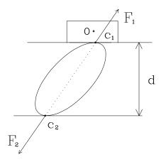
Figure 4: Contact points and contact forces in the manipulation process.
