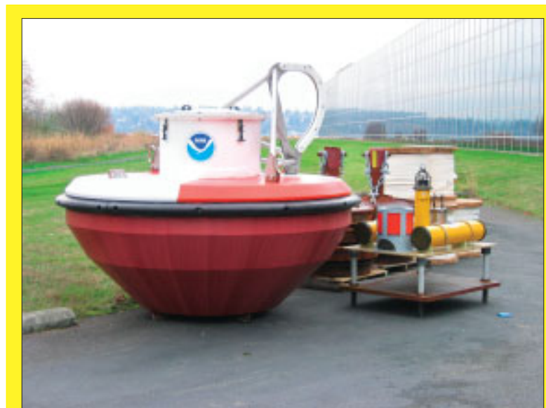
OH BUOY! A second generation Deep Sea Tsunami Detection Equipment (DART-2) buoy, similar to the one that will be deployed in the Indian Ocean near the Andaman & Nicobar islands.
