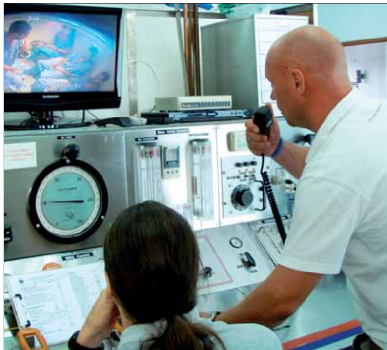
The control panel outside of the chamber has many redundancies to ensure the safety of patients. Photo: Sea Bees
