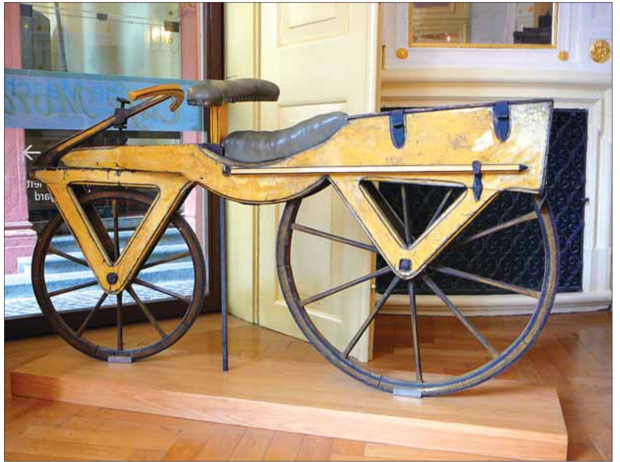
The laufmaschine designed by German Baron Karl von Drais; pedals and crank came later. Photo: Gun Powder Ma
