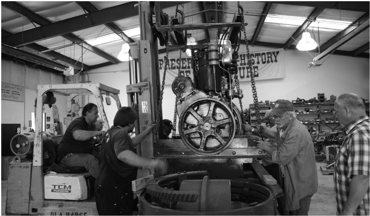
In April 2013, tractor restoration volunteers and museum maintenance staff mount the restored engine onto the 1919 Holt 75 tractor frame.
