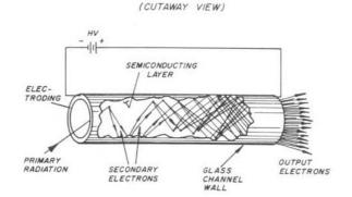
Fig. 2. A straight channel electron multiplier.
