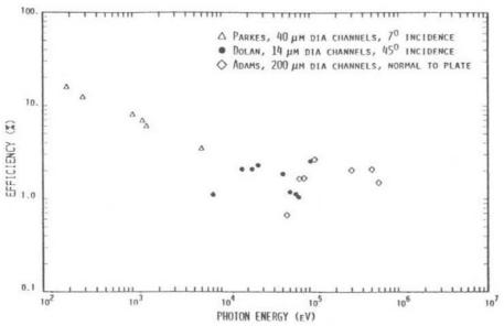
Fig. 11. X-ray detection efficiencies from ref. 3.
