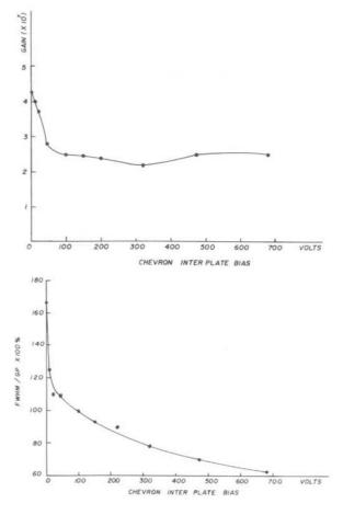
Fig. 7. (a) Gain vs interplate bias voltage for a Chevron at 150  $\mu$ m plate separation. (b) Normalized full width at halfmaximum (fwhm/G<sub>P</sub>) x 100% vs Chevron interplate bias voltage.
