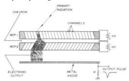
Fig. 5. Chevron operation (Side view).
