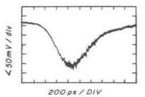
Fig. 12. Sampling oscilloscope trace of Chevron (200 V interplate bias) output pulses. Signal was derived from a 50  $\Omega$  conical anode.
