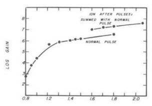
Fig. 8. Gain vs voltage characteristic for a Galileo high gain curved channel plate.
