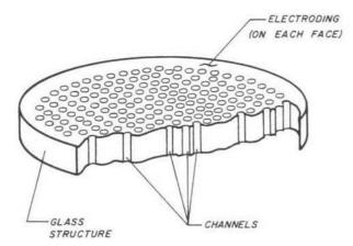
Fig. 1. A microchannel plate, (cutaway view)
