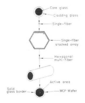
Fig. 9. Etchable core MCP manufacturing process.
