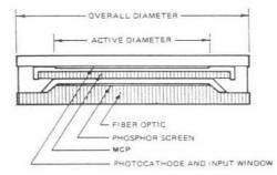
Fig. 15. A proximity focus image intensifier tube.
