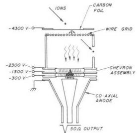
Fig. 18. A Chevron "start" detector (adapted from ref. 66).
