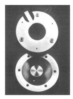
Fig. 13. Chevron and 50  $\Omega$  anode.
