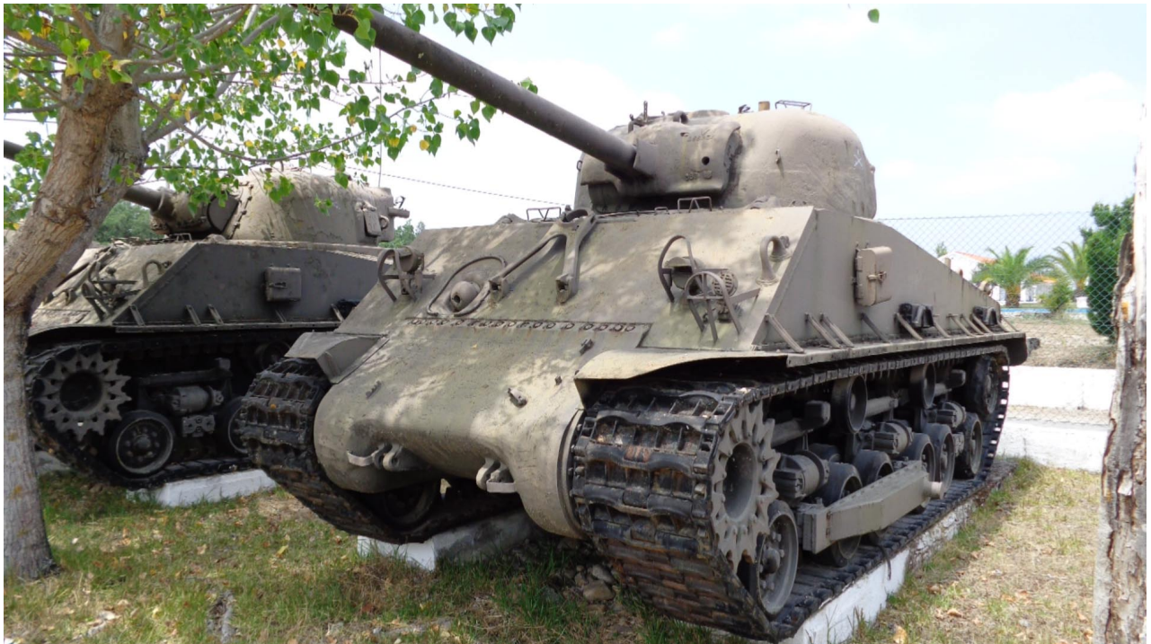
M4A3E4(76) HVSS Sherman Dozer – Campo Militar de Santa Margarida (CMSM) Santa Margarida da Coutada (Portugal) Serial Number 74470, was built as an M4A3(105) HVSS
