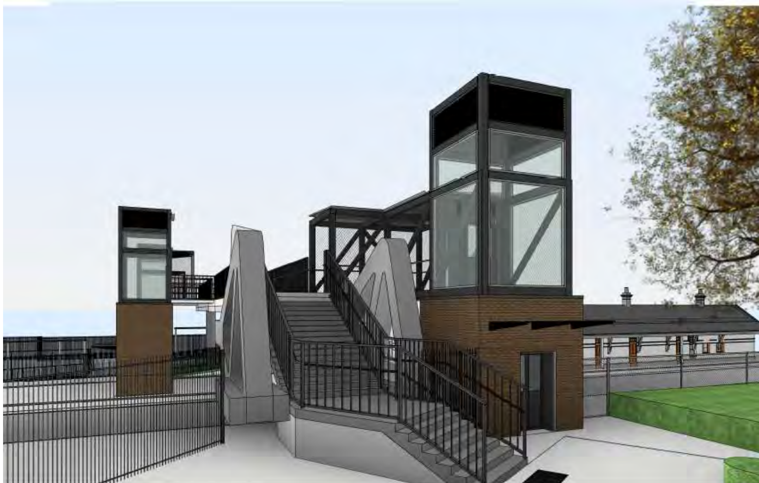
Figure 30. Design Projection (view to north-west) of the arrangement of the stairs and lift at the Queen Street end of the overhead bridge. (Source: Transport for NSW)
