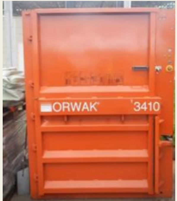
Fig. 16. Press compactor for packaging materials
