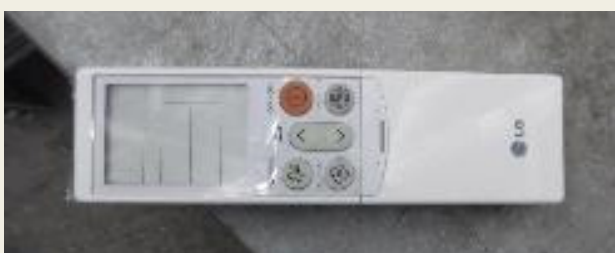
Fig. 35. Fan coil control panel
