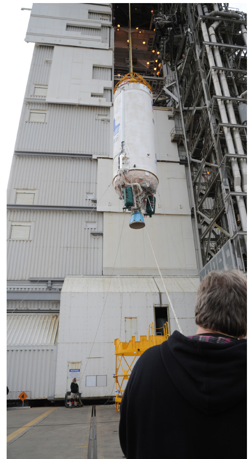
(10/09/2012) --- VANDENBERG AFB, Calif. – A Centaur upper stage is lifted onto the first stage booster of a United Launch Alliance Atlas V at the launch pad at Space Launch Complex-3E at Vandenberg Air Force Base, Calif. in preparation for the launch of the Landsat Data Continuity Mission.
