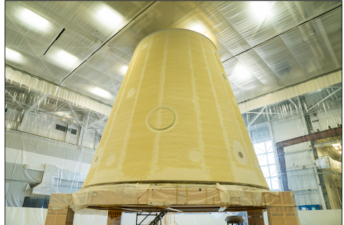
Thermal Insulation Application Complete on LVSA
