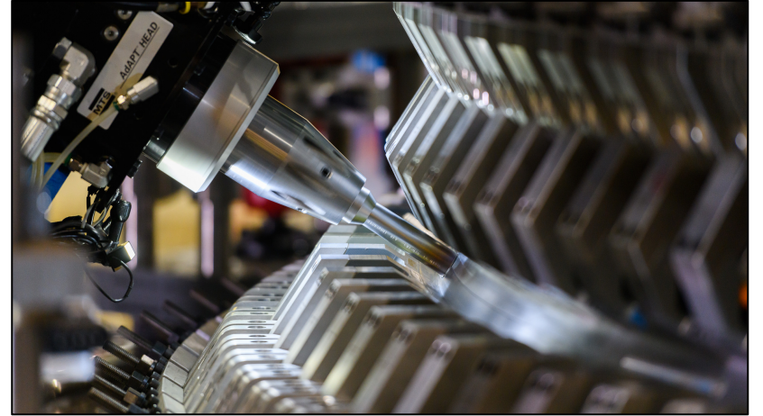
EM-2 Close-Out Welds at MAF
