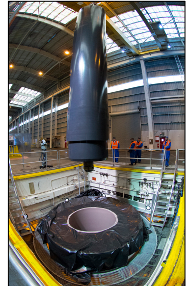
Engineers remove the core after casting the booster case with propellant
