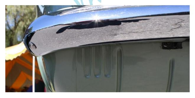
The original 1960 Corvair design called for the horn to be behind the slots under the passenger front bumper and in front of the tire. Records indicate that a change was made in April 1959 to move the horn up to a safer location behind the headlight buckets.
