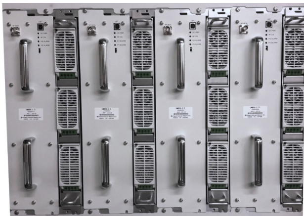
Figure 36: 4 Amplifiers In Parallel With Associated Power Supplies
