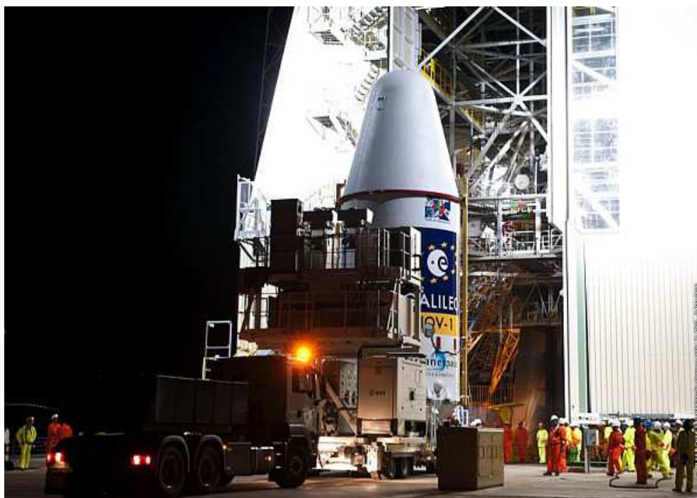
Figure 6.2.3.2.2b – Arrival of upper composite in the mobile gantry
