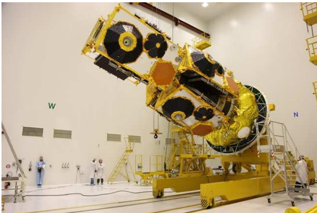
Figure A4b 1-2 Nose block with Globalstar 2 dispenser ready for Fairing encapsulation
