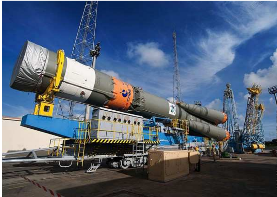
Figure 6.2.3.2.2a – LV transfer from the assembly building (MIK) to the launch pad
