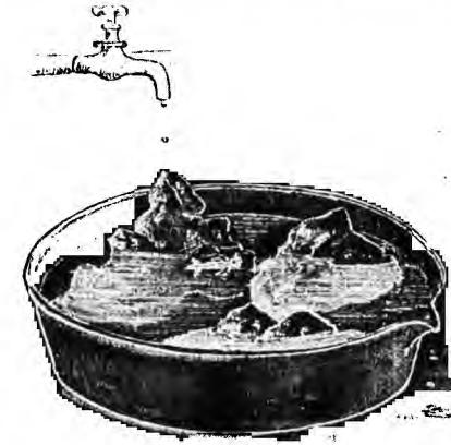
Fig. 188. Pan for rearing rock or bottom-dwelling larvae ( \times \frac{1}{2} ). Original drawing by P. Tillyard.
