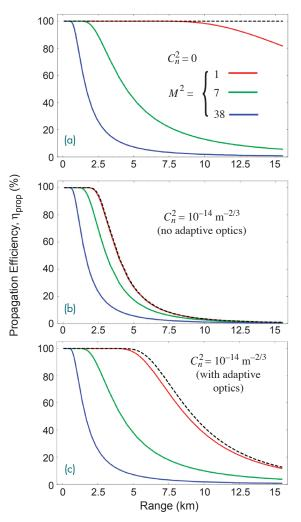
Propagation efficiency versus range for incoherently combined fiber laser beams with beam quality parameters  $M^2 = 1$ , 7, and 38: (a) in vacuum, (b) in a turbulent atmosphere with  $C_n^2 = 10^{-14} \text{ m}^{-2/3}$ (no adaptive optics), and (c) in a turbulent atmosphere with adaptive optics. Laser parameters are listed in Table 1. The dashed curve represents the theoretical upper limit for coherent and incoherent combining.
