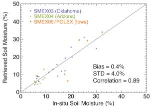
FIGURE 11 WindSat solid moisture validation against SMEX data.
