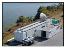
The W-band Advanced Radar for Low Observable Control (WARLOC) is a 94-GHz, high-power, coherent mmW radar.
