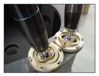
FIGURE 9 Piezoelectric screw-drive actuators for control of hexapod secondary ring.
