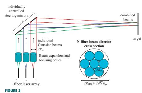
Schematic diagram of incoherently combined fiber laser beams directed to a target.
