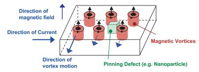
A schematic diagram illustrating the concept of pinning of the vortices by nanoparticles embedded in the superconductor.
