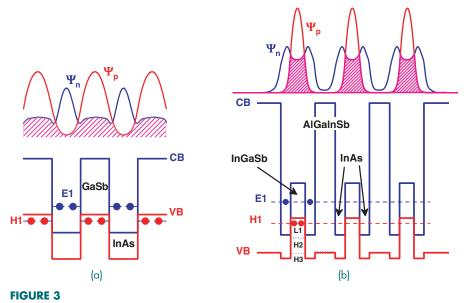
(a) Simple T2SL and (b) WSL heterostructures and wavefunctions.
