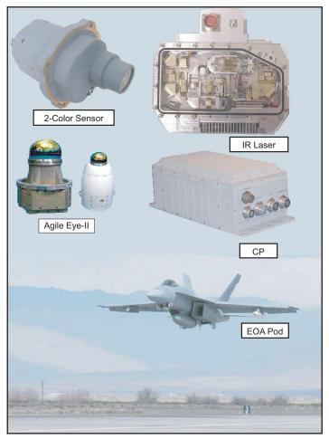
**FIGURE 4** TADIRCM components and the EOA pod.
