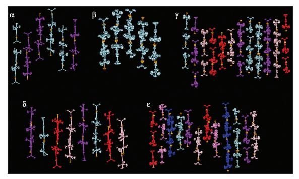
Relationship between the layers in polymorphs of picryl bromide. In each image, crystallographically unique layers are depicted in a different color. Bromine atoms are shown in orange to help orient the individual molecules.
