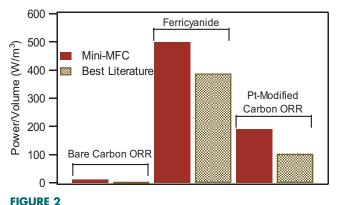
Power density per volume for the mini-MFC compared to best literature values for three cathode reactions. ORR = oxygen reduction reaction
