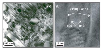
(a) A bright-field TEM image near the [001] zone of the superconducting matrix showing nanoparticles embedded in the matrix for a Ho-doped YBCO sample (lower Ho concentration than specimen of Fig. 5). Note the (110) twins. (b) HRTEM image showing the (110) twins. Note the apparent bending of twins close to the particle. Such bending could result from the interaction of strain fields present close to the particle and the twins.
