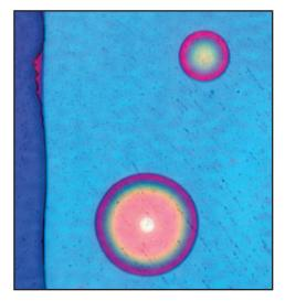
**FIGURE 9** Optical micrograph of the SC diamond domes. The smaller dome is 9.2 microns in diameter.
