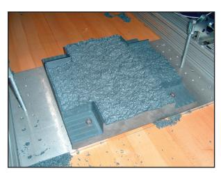
Fabrication of rough surfaces for acoustic analysis.
