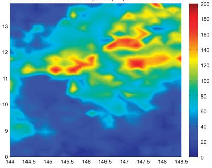
Forecast STD of acoustic coverage area (km<sup>2</sup>) at 125 Hz 2007081000
