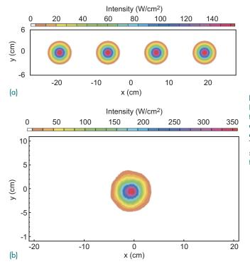
HELCAP simulation showing a time-averaged transverse intensity profile of laser beams at (a) the source and (b) incoherently combined on target at a range of 1.2 km. The atmospheric turbulence level used in the simulation is the same as those measured in the experiment.
