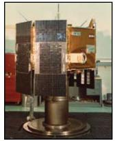
Navigation Technology Satellite-2 (NTS-2) was the first operational NAVSTAR GPS satellite.
