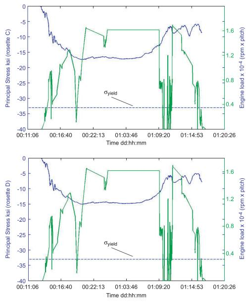
Principal stresses recorded during the trip from rosettes C and D. Also shown is the yield stress for the deck material. Note that the largest stresses began near sunset on 6/7/07 and ended about sunrise on 6/8/07. Stress correlates well with engine load.
