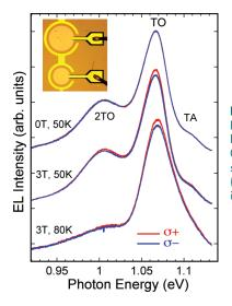
Electroluminescence spectra from the Si *n-i-p* structure with the Fe/Al2O3 contact at 50 K and 80 K, and at magnetic fields of 0 T and 3 T. The inset shows an optical photograph of the LEDs studied. Spectral peaks corresponding to transverse acoustic (TA) and transverse optical (TO) mediated recombination are identified in the figure.
