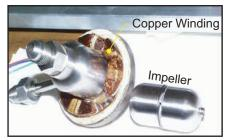
bly and an external motor drive. Permanent magnets embedded in the impeller are magnetically coupled to the motor drive (located on the outer surface of the pump housing), which in turn rotates the impeller. Hence, like other magnetically driven pumps, the ABI pump does not need a driving shaft between the motor and the impeller. This allows the fluid system to be hermetically sealed from the surrounding to mitigate fluid leakage.
