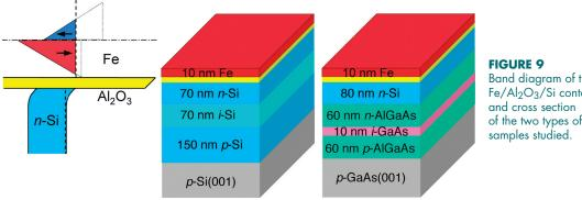
FIGURE 9 Band diagram of the Fe/Al<sub>2</sub>O<sub>3</sub>/Si contact and cross section
