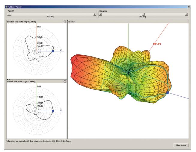
Representative display of a CMAST antenna pattern that includes the effect of the surrounding platform.
