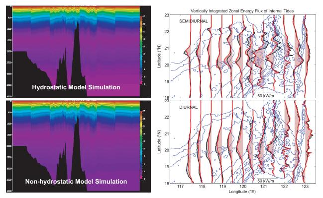
Simulations of the internal-wave generation and propagation with hydrostatic and non-hydrostatic models (left). The energy flux of the internal tides (right); red and black correspond to results with and without west ridge blocking, respectively.
