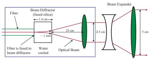
Schematic diagram of fiber output coupler and beam expander.
