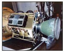
TIMATION I (rectangular object in center of photo) was successfully tested in a "piggyback" launch aboard an Air Force Thor-Agena D.
