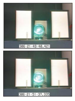
Two CCD camera images of four beams incoherently combined on target (10 cm radius power meter) at a range of 1.2 km. The first panel shows the combined beams at ~180 sec and the second image is at ~300 sec. The later image shows the four individual beam centroids randomly displaced by ~4 cm due to atmospheric turbulence.
