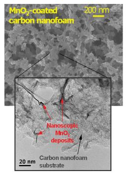
Scanning electron micrograph (top) and transmission electron micrograph (bottom) of a MnO<sub>2</sub>-carbon nanofoam hybrid nanoarchitecture.
