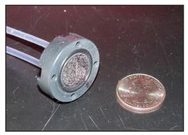
FIGURE 1 NRL's mini-MFC (anode chamber shown).
