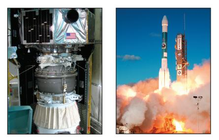
Left photo: Upper Stage spacecraft attached to Star48 3rd stage of Delta II 7925 booster. Right photo: MiTEx/Upper Stage launch, 21 June 2006, 2215Z. (Courtesy USAF)
