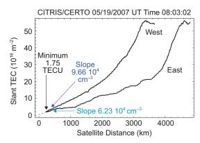
Measurements of total electron content (TEC) on the west and east side of the point of closest approach. Determination of absolute TEC uses extrapolation to zero separation between beacon and receiver satellites. The electron density is estimated from the derivative of the TEC with intra-satellite distance.
