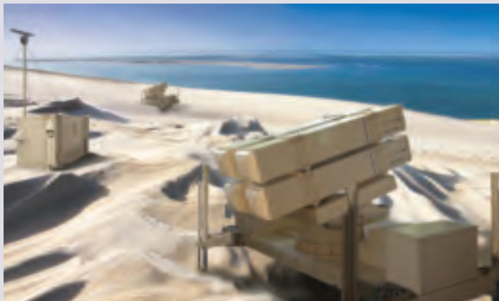
Artist's impression of the coastal defence battery featuring two quadruple Marte missile launchers and a remote radar shelter
