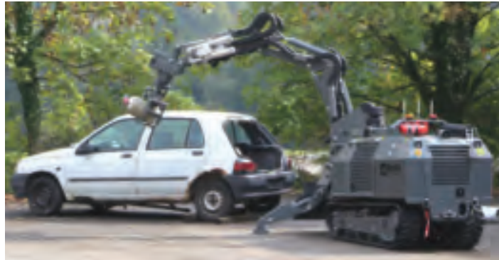
The MW50 demonstrates its ability to handle a vehicle-carried IED
