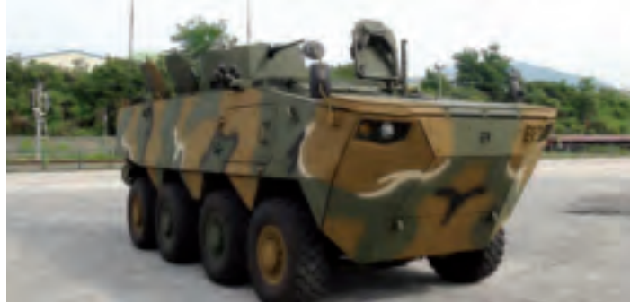
Latest Hyundai Rotem KW2 (8x8) in baseline APC configuration, armed with a roof-mounted .50 M2 HB machine gun
