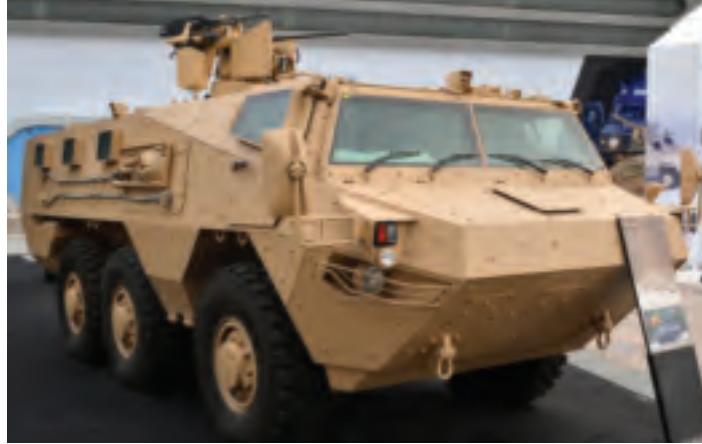
VAB Mk III (6x6) at IDEX 2015 fitted with the Kongsberg remote weapon station armed with a .50 heavy gun and a 7.62mm MG
