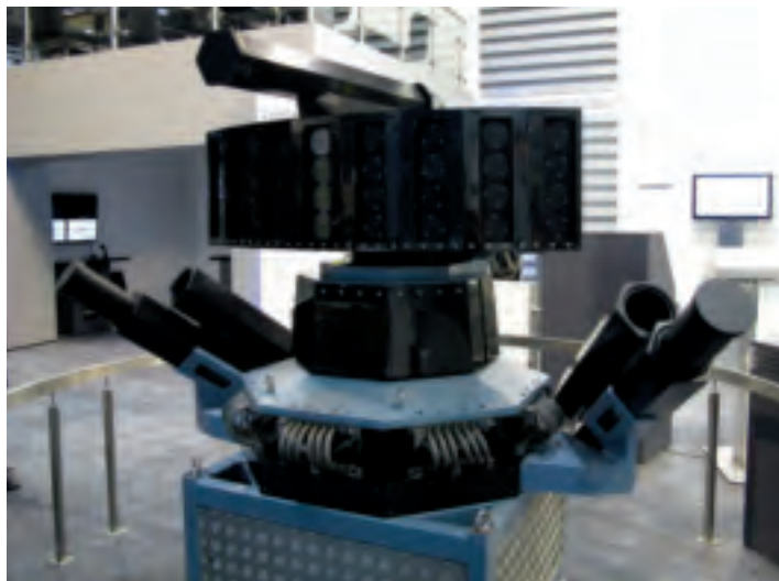
The MASS decoy system is being enhanced so as to provide better protection against both anti-ship missile threats and torpedoes
