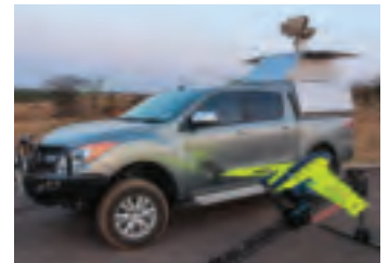
Top: mobile surveillance system (solar power panel still to be deployed); above: customised pickup with Will-Burt mast and FLIR sensor suite alongside Desert Wolf's Bat UAS on a launcher
