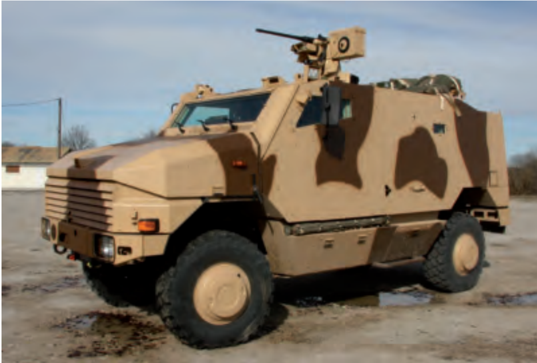
Aravis (4x4) protected vehicle armed with a Kongsberg Protector RWS armed with a .50 M2 HB MG
