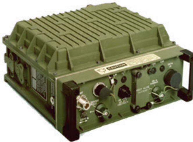
Figure 6-1. EPLRS Vehicle-Mounted Radio.
