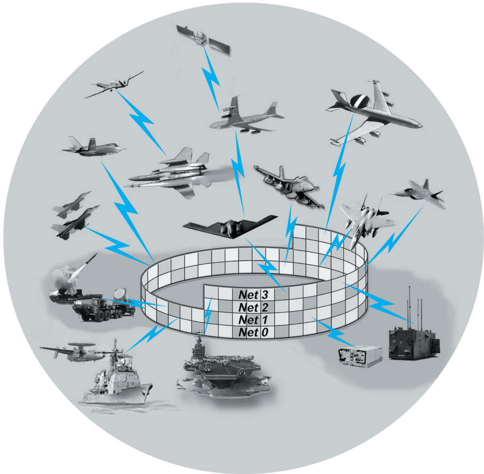
Figure 2-5. JTIDS units automatically transmit, receive, and relay data at pre-assigned times on pre-assigned nets based on instructions given to their terminals when they are initialized. These pre-assignments are determined in advance of operations to support the expected information exchange requirements of the force.
