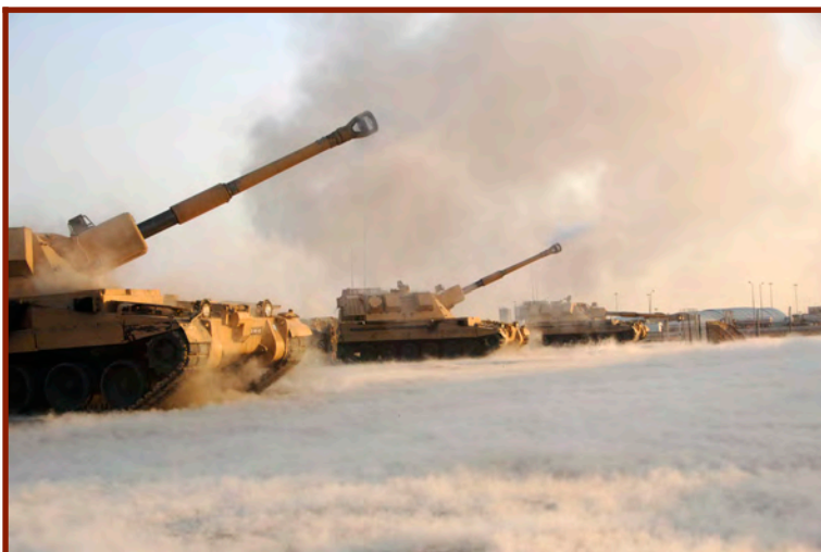
Fig. 2. AS90. British soldiers from J Battery, 3rd Regiment, Royal Horse Artillery fire rounds to calibrate their AS90 155 mm self-propelled guns in Basra, Iraq, Aug. 28, 2008
