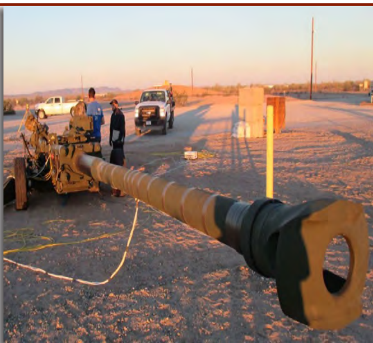
Fig. 7. Show Caption + Morning pre-fire checks and daily preventative maintenance on the Extended Range M777A2 before testing
