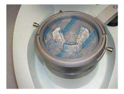
Figure 5: The Erkoloc-pro occlusal guard following forming as it goes through the cool down cycle.
