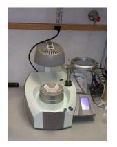
Figure 1: Erkoform computerized "Sudden Vacuum" pre-charged pump chamber former from Glidewell Labs.
