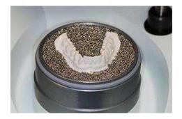
Figure 2: The model to be treated is placed in the base filled with metal shot and the shot is placed to only expose the area that will be captured in the material.
