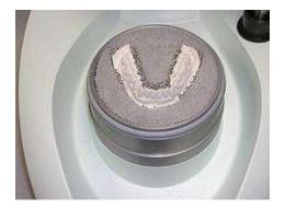
Figure 3: A sheet of premade blockout is placed over the cast to cover the shot beyond the model.
