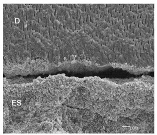
Figure 11: SEM demonstrating microgap formation with AH-26 epoxy sealer due to polymerization shrinkage. (ES – epoxy sealer, D – dentin)
