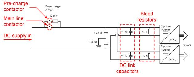
Figure 5: Simplified electrical schematic for Class 455 IGBT propulsion, showing equipment for two traction motors
