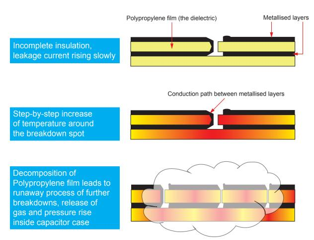
Figure 7: Drawing illustrating failure of self-healing
