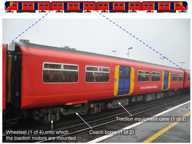
Figure 4: Class 455 unit and Motor Open Standard coach. Photograph is not of the unit involved in the accident
