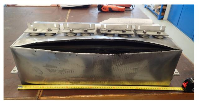
*Figure 8: The damaged capacitor removed from coach 62826 prior to examination at Electronicon's facilities in Germany*
