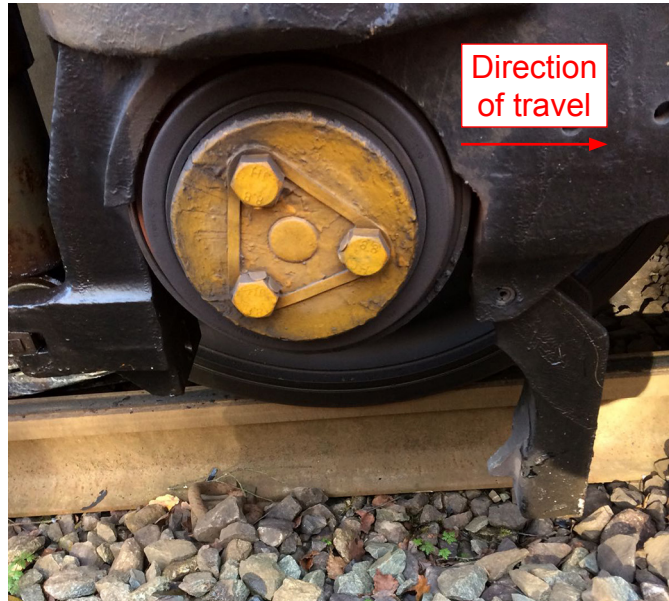
Figure D12: Wheelset lift bracket at wheel position 5 hanging down after the accident (courtesy Network Rail)
