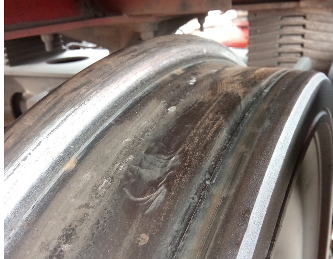
Figure D5: Flat on wheel at position 8 (courtesy DB Cargo)
