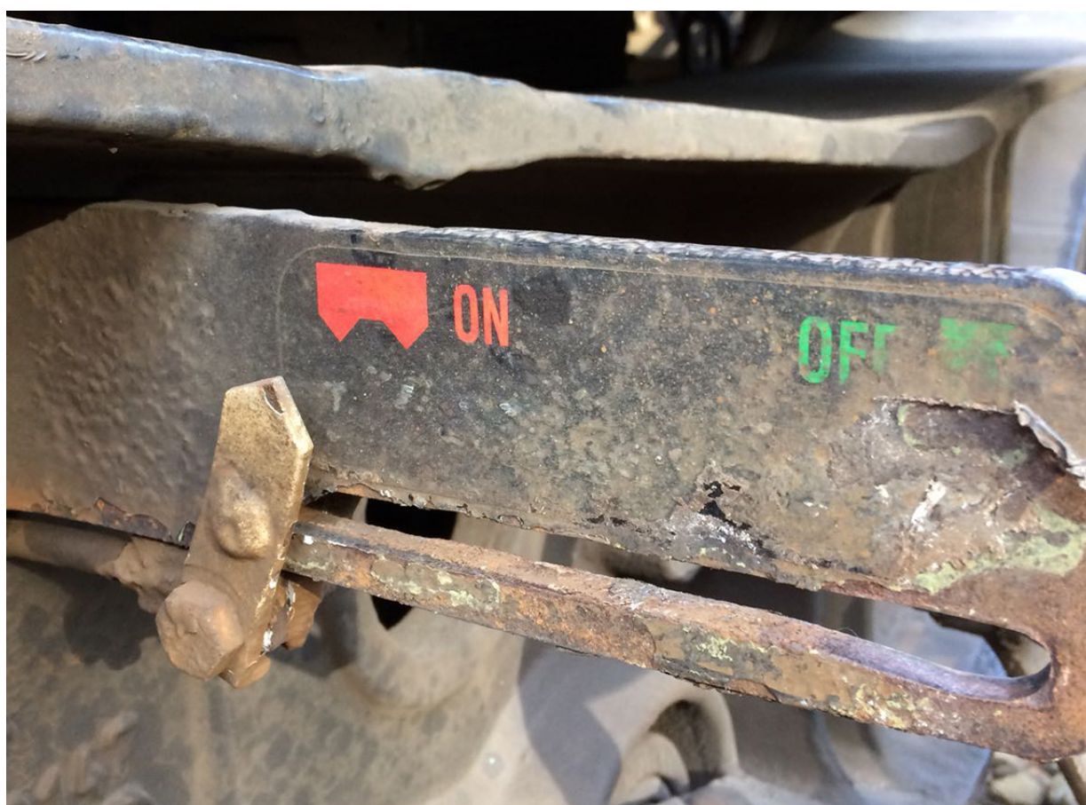
Figure 17: Handbrake indicator on wagon GERS89009 after the accident (courtesy Network Rail)
