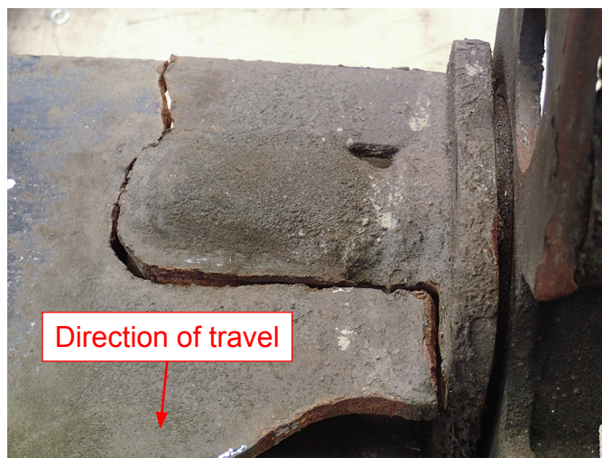
Figure D3: Cracking of slave brake beam at wheel position 8
