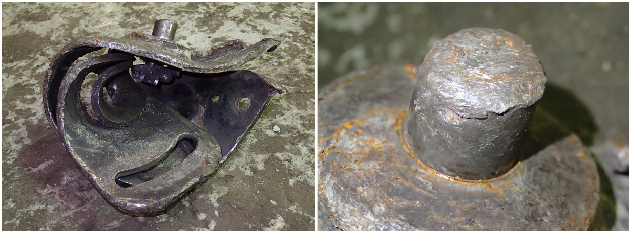
Figure D10: Remains of block holder from wheel position 6 and close up of fractured hanger pin
