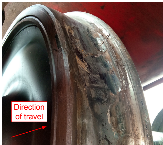
Figure D4: Flat on wheel at position 5 (courtesy DB Cargo)
