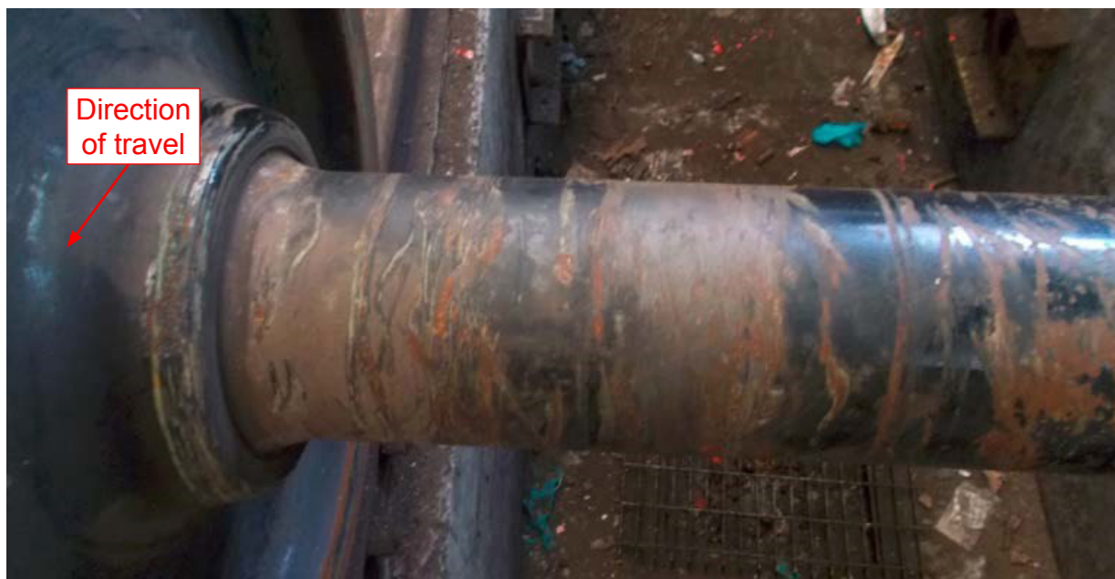
Figure D13: Evidence of rubbing contact adjacent to wheel position 5 (courtesy DB Cargo)
