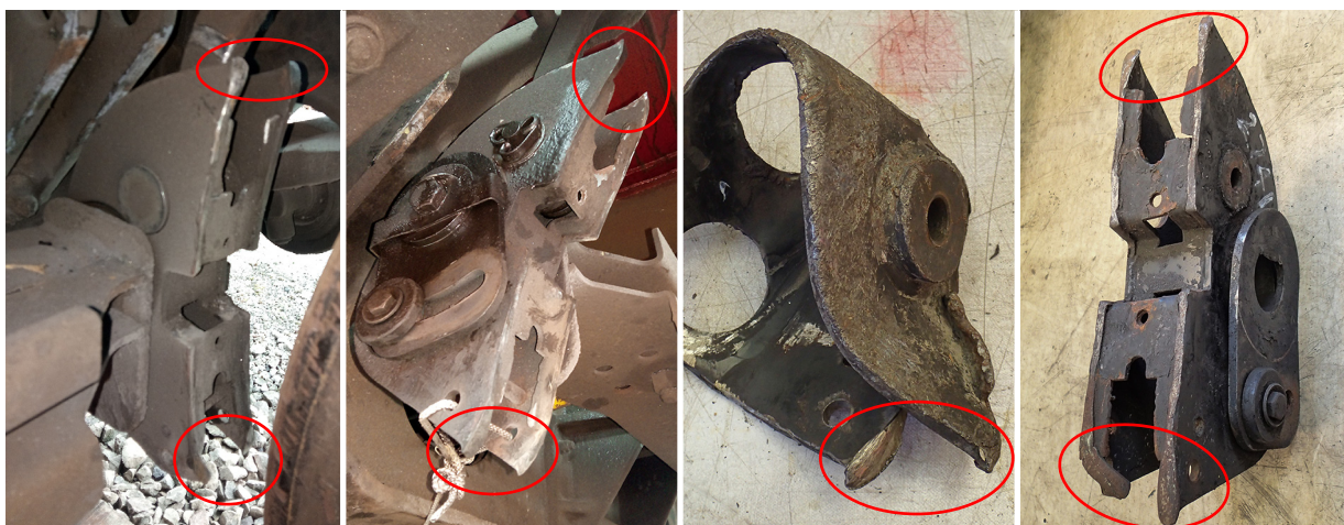
Figure D7: Brake block holders from wheel positions 8, 7 (both courtesy DB Cargo), 6 and 5 with worn corners indicated
