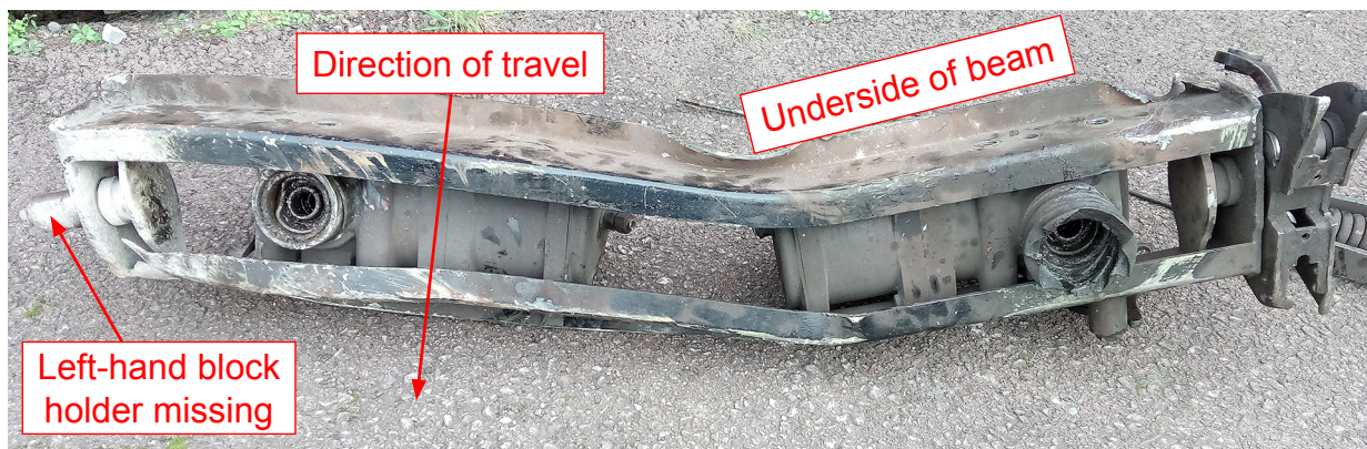
Figure D2: Master brake beam from bogie 2741 (courtesy DB Cargo)
