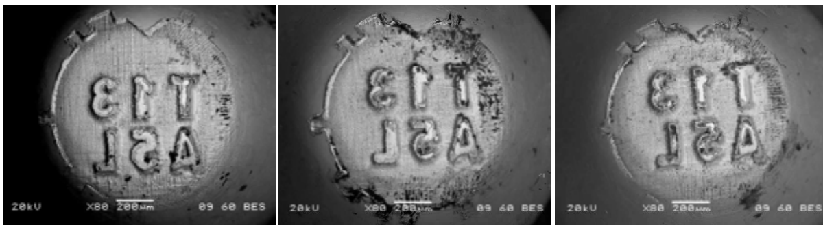
Figure 6: SEM backscattered images of three pins microstamped for the Taurus firearm.
