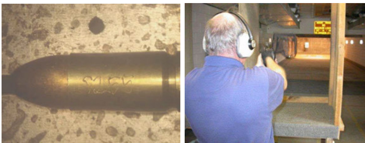
Figure 2: a) Unfired cartridge with inscribed identifier. b) Firing in progress with catch-basket.
