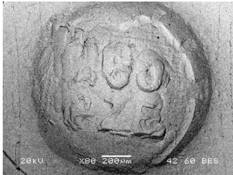
Figure 5: Cartridge #H519, PMC ammunition, Hi-Point handgun
