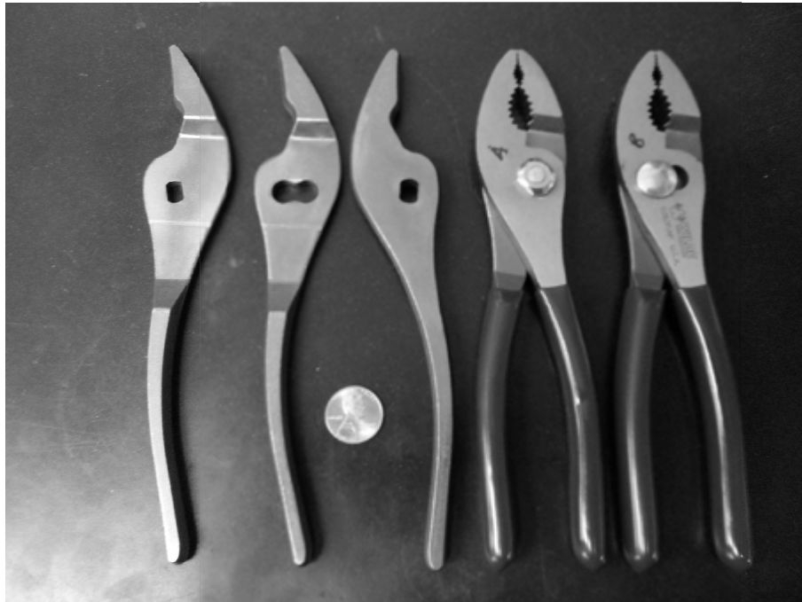
Figure 1: Slip joint pliers in their unfinished and finished states. From left to right: plier halves (single and double hole) before broaching; an example flat side of pliers that will be polished; finished and labeled pliers (sides A and B).
