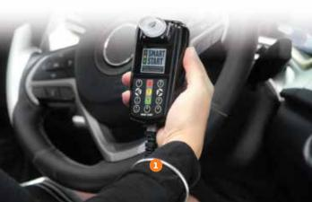
If you qualify to participate in the program, an ignition interlock device will be installed in your vehicle. The device is designed to stop a vehicle from starting or operating when the driver has been drinking.
