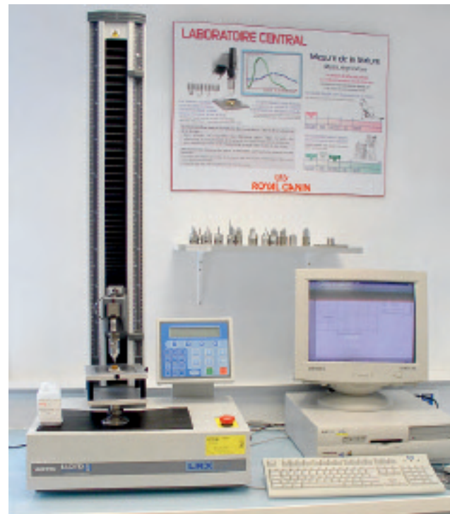
The texturometer is used to measure the kibble's resistance to the force of the cat's teeth and jaws. Interchangeable modules imitate the shape and size of teeth according to the size and age of the cat.
