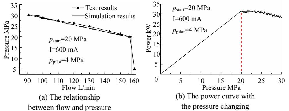
Fig. 11 Constant power characteristics at  $p_{start}=20\text{MPa}$
