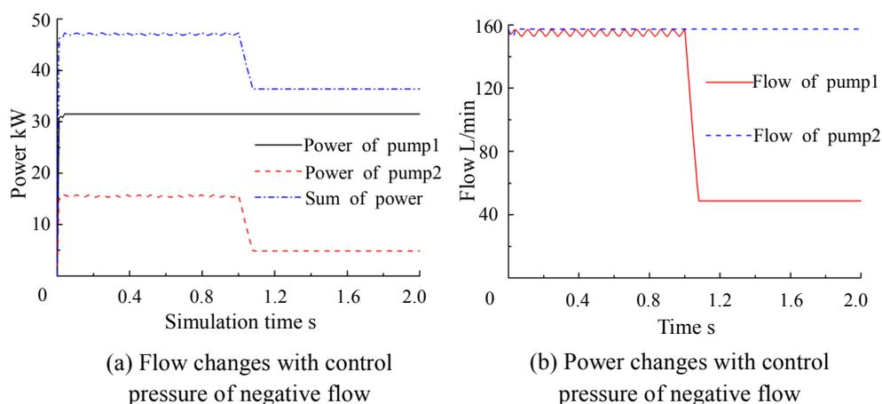
Fig. 13 Results of sensing control of negative flow in cross power control
