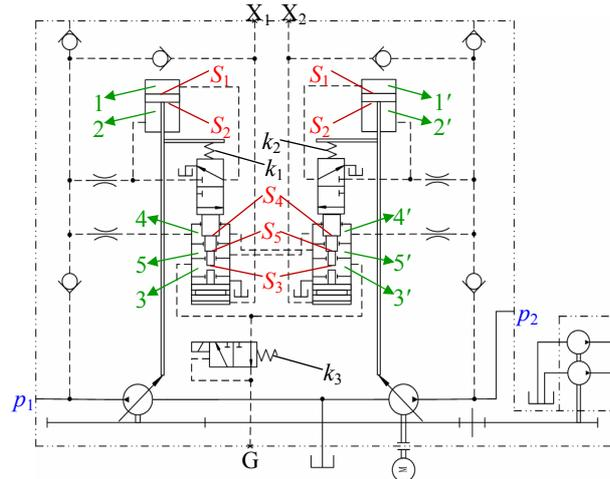
Fig. 2 Principle of cross power control system
