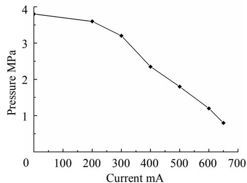
Fig. 9 The relations hip between the pilot pressure and current of proportional valve
