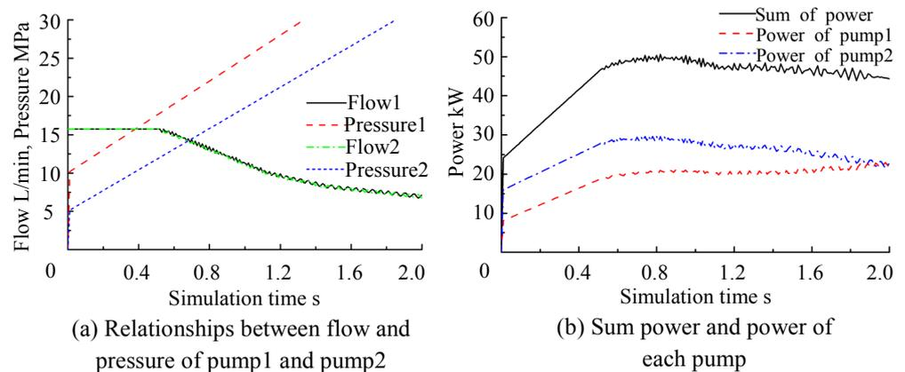
Fig. 12 Characteristics of the cross power control with different output pressure ( $p_{1start}=10\text{ MPa}$ ,  $p_{2start}=20\text{ MPa}$ )
