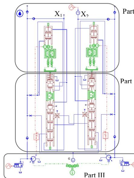
Fig. 8 Model of the double pump with cross power control
