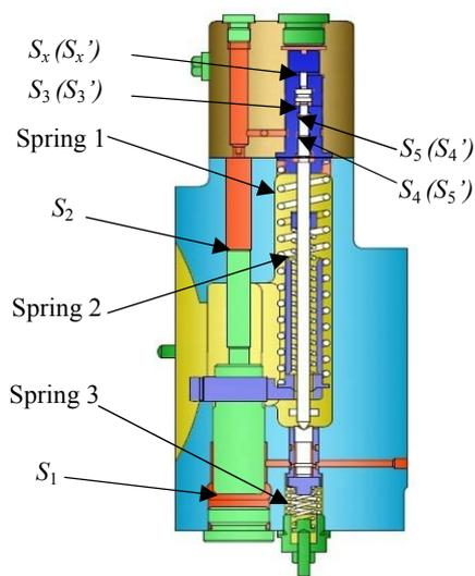
Fig. 7 The displacement changing mechanism
