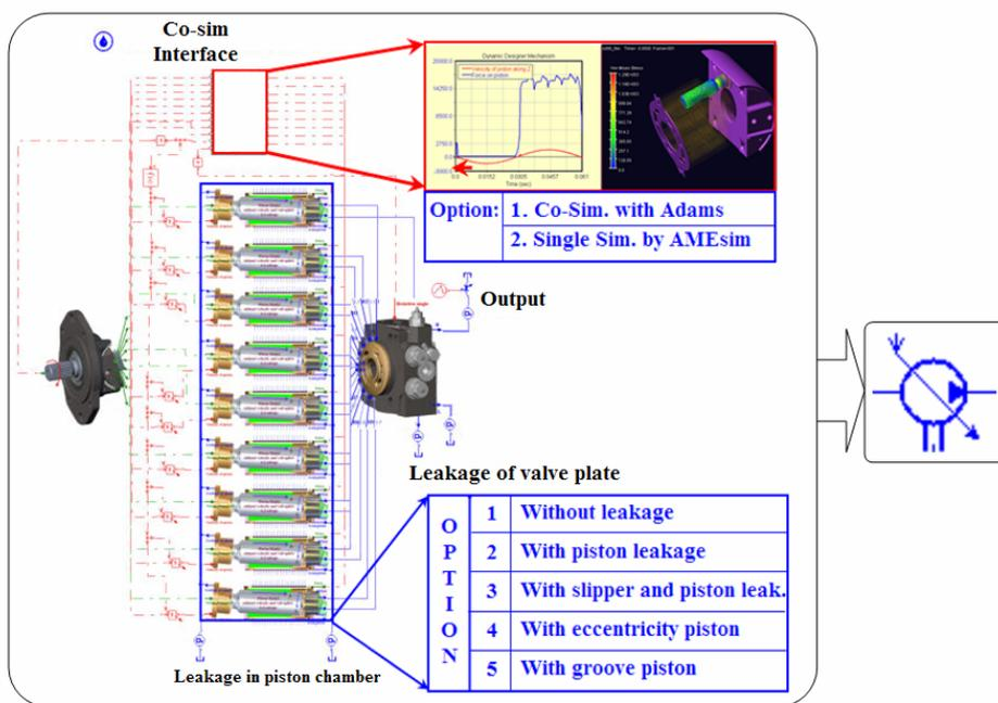
Fig. 6 The whole hydraulic model of the pump
