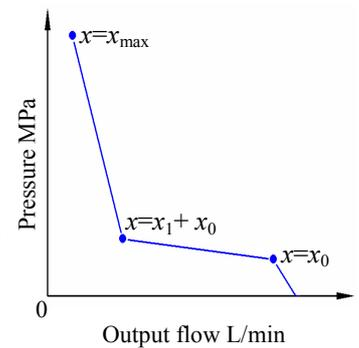
Fig. 3 The relationship between the output flow and pressure of individual pump
