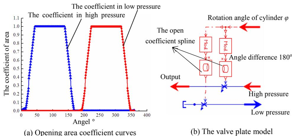
Fig. 5 The model of valve plate
