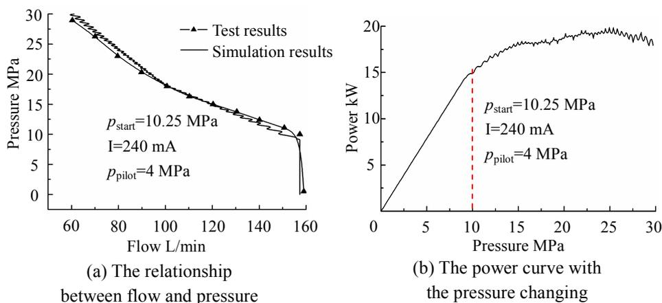
Fig. 10 Constant power characteristics at  $p_{\text{start}}=10.25\text{MPa}$
