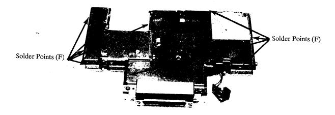
NOTE: When replacing the shields, make sure the flanges from the top shield (the shallow one) overlap the flanges from the bottom shield on either side of the expansion bus port.
