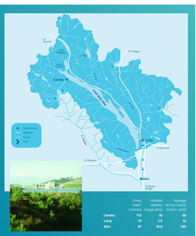
\* The 'head' is the difference in height between the water supply feeding the power station and the turbines.
