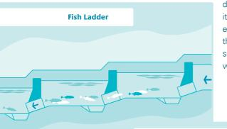
There are two types of fish pass, the fish ladder and the fish lift, known as the Borland lift.
