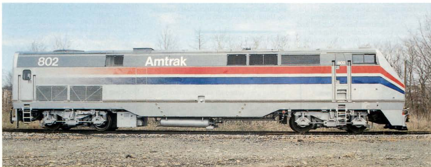
If you plan on riding the California Zephyr , Sunset Limited , or City of New Orleans soon, chances are you will ride behind Amtrak's General Electric AMD103s. The new 4,000 h.p. locomotives were a cooperative design venture between Amtrak and GE. New features include office-environment cabs, non-curved aerodynamic styling, and a 2,200-gallon fuel tank built as an integral part of the frame. Photo courtesy of GE
