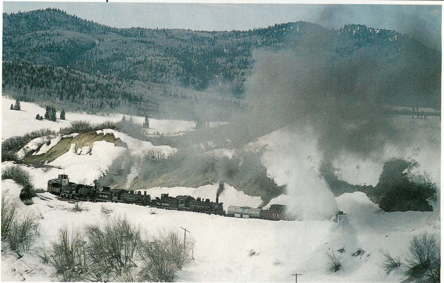
There was quite a show along the Colorado/New Mexico state line this spring when Cumbres & Toltec Scenic Railroad called out steam-powered rotary OY to clear its line up to Cumbres Pass. The drifts—up to 21 feet deep—remaining after the long Rocky Mountain winter were a stiff challenge for the OY, fortified by a tripleheader of Mikados 487/497/488, shown at work on May 3, 1993. Steve Brown
