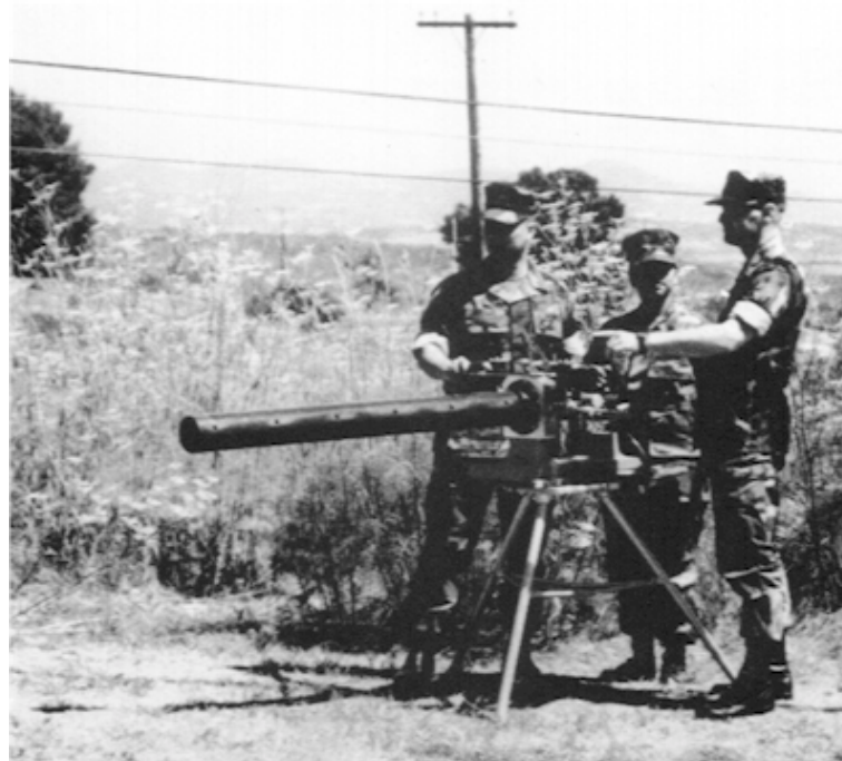
Figure 15. The US Marines test a unidirectional acoustic infrasonic weapon developed by SARA.
