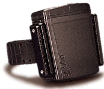
Figure 2. Photograph of a transmitter bracelet
