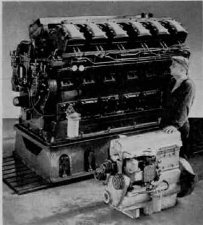
A comparison in size between the smallest and the largest Cummins Diesel.
