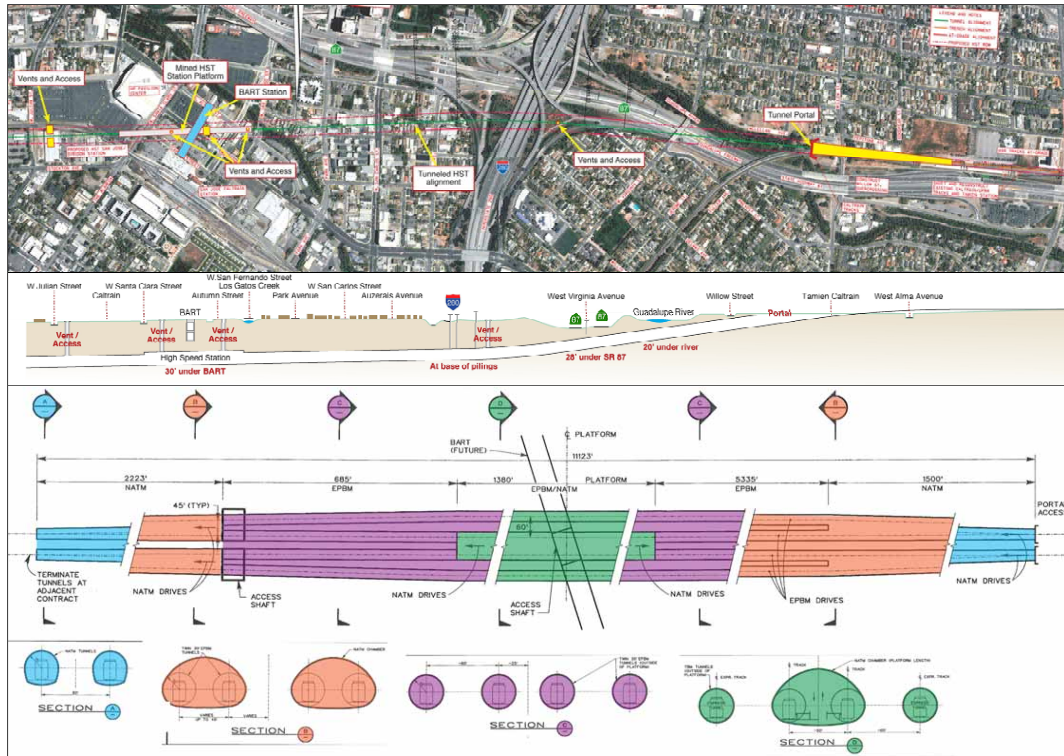
Figure 6. Plan & Profile and Track Configuration for "Deep Tunnel" Option
