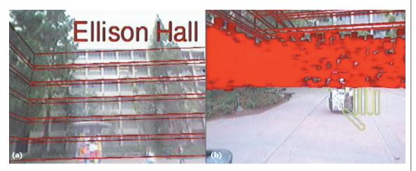
**2** (a) Augmented reality view of one of the two buildings for which we built models. (b) Visualization of spots with "insufficient wireless" signal strength. The density of the data prohibits discerning differences in the data intensity.
