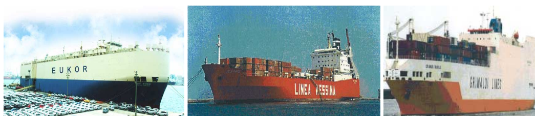
PCTC, a Ro-ro combined vessel a modern ro-ro/container vessel with PCC inspired design
