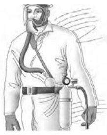
Full Facepiece Supplied-Air Respirator (SAR) with an auxiliary Escape Bottle APF=1,000 APF = 10,000 (if used in "escape" mode) Needs to be fit tested
