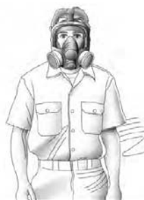
Full facepiece (Elastomeric) APF=50 Needs to be fit tested
